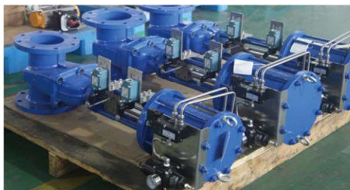
Linear actuators mounted to flanged gate valves prior to dispatch.
