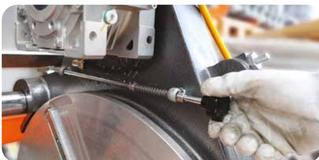
Milling Cutter with fast removing system
