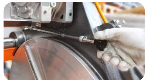
Milling Cutter with fast removing system
